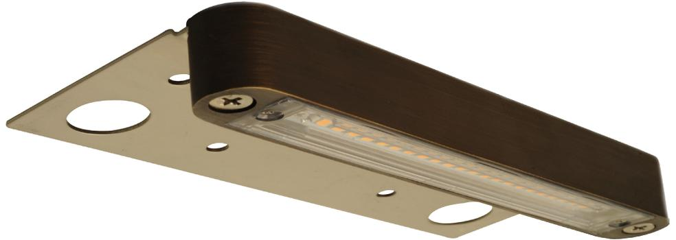
Crafted from cast brass, the Cascade hardscape light features a highly efficient embedded 4-watt, warm-white LED array (251 lumens). It can be mounted under a horizontal cap or flush to a vertical or horizontal surface. Clear high-impact lens. Five-foot factory-installed 18/2 wire lead.
