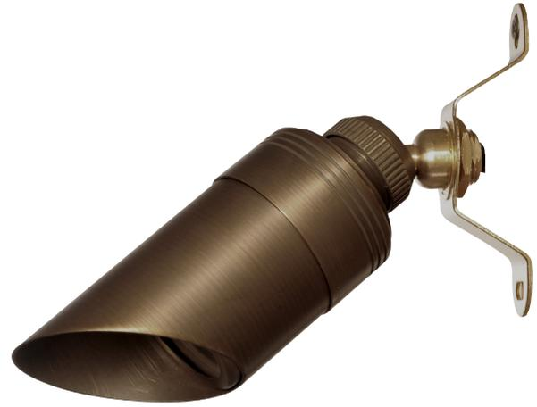
The small Cypress down light features an angled shroud from which a narrow or broad lamp can spread its light, precisely aimed by virtue of a locking orbital pivot. Shroud is adjustable in-and-out for beam control, and sealed by three O-rings. Y-bracket mount included.
